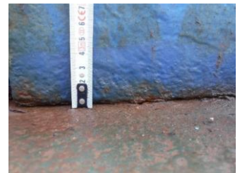
Panel to coaming clearance zero
