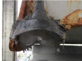
Packing rubber with permanent imprint
