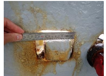
Measuring longitudinal clearance
